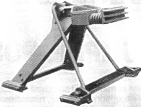
Transit cars pose special problems. Structural strength, coupling mechanisms, appurtenances and car-end configuration are varied and usually quite unlike freight car design. This transit car Bumping Post has an extra-length, spring-loaded face that will clear car equipment. The face is also equipped with anti-climber ribs to help prevent the car from riding up if the bumper is hit too hard.
