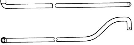
Connecting Rod for Target Stand and Sliding Derail: this is a 3/4 inch rod made as shown here.
